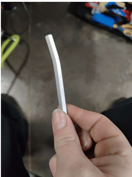
A picture of a standoff from a long-range catapult after one shot. A picture of a modified catapult to withstand the force of the rubber bands.
